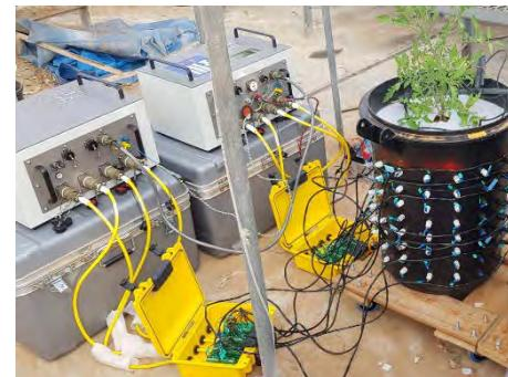
**Figure 2:** The lysimeter system during an electrical survey.
