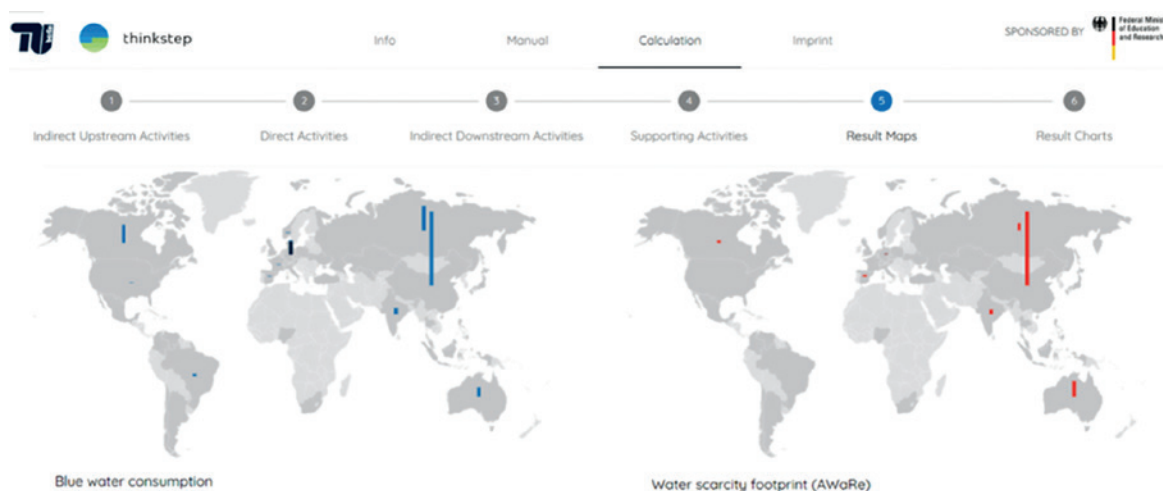
Figure 1: Regional water consumption (blue bars) and resulting local impacts (red bars) caused by a company at its production site (Germany) and along its global material supply chains determined by the free OWF online tool (© WELLE OWF tool, TU Berlin).
