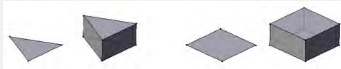
Extrusion of a triangle and a quadrilateral.
