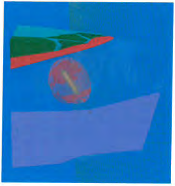
Temperatur field of a drift charged with 20 POLLUX containers 200 years after emplacement (red: 50°C iso-surface)
