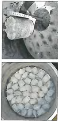
Layer of Rock Salt Compacts Binary Mixture after Oedometer Test at 5 kPa
