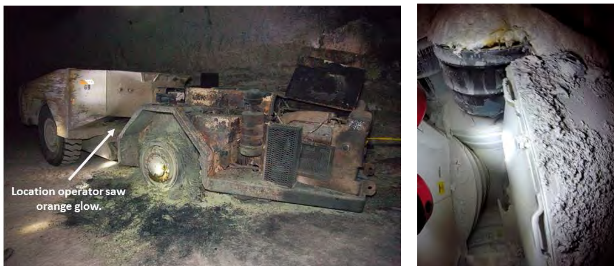
Figure 3-1. WIPP operational accidents: Salt haul truck fire (left) and radiological release (right).
