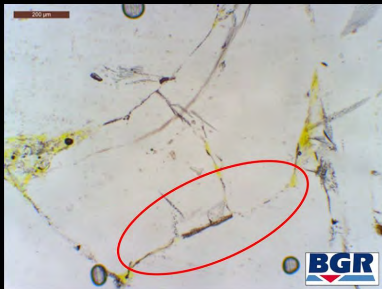
Pressure solution in compacted crushed salt (oedometric compaction; 50°C, max. 30 MPa)
