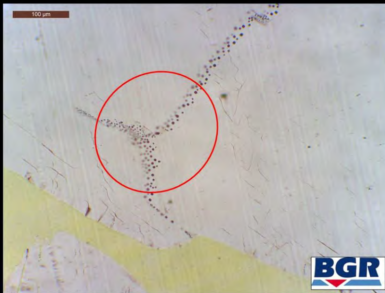
Fluid inclusions in crushed salt raw material
