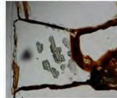
Magnified sections: visualization of penetration into rock salt
