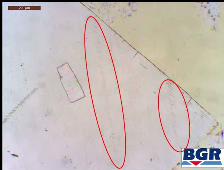
En-échelon structures in crushed salt raw material
