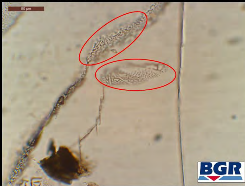
Fluid inclusions (oedometric compaction; 50°C, max. 30 MPa)
