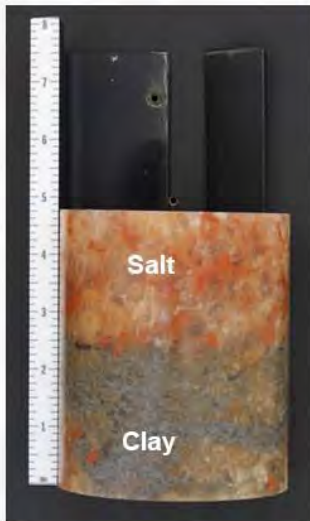
Salt/clay interface Fracture shown is typical of all tests
