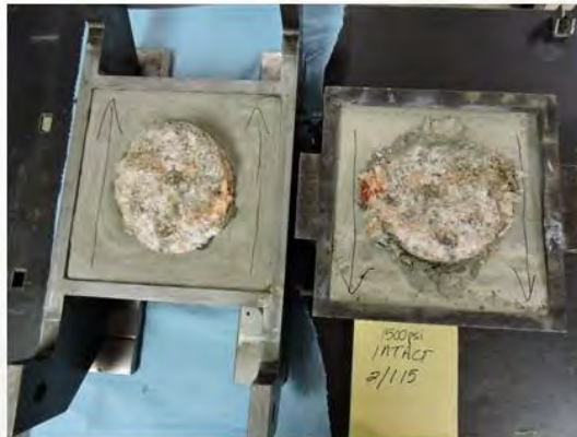
Intact test, \sigma_n=1500 psi (10.3 MPa); salt crystals cross through interface
