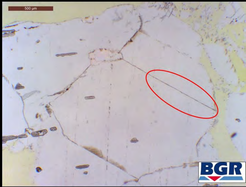
Microcracks in crushed salt raw material
